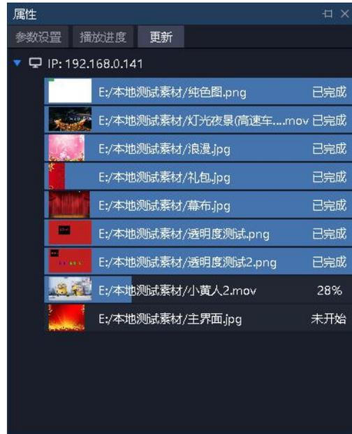
Display the file transfer status when the media files are synchronized online and offline, which is convenient for users to view the files that are being synchronized, not started, or failed to synchronize, and understand whether the transfer is complete.
