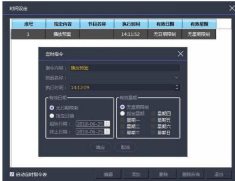
Add a timing switch command through "New", as shown in the pop-up window in the middle of the picture above, you can set which time period and time to play which plan.
