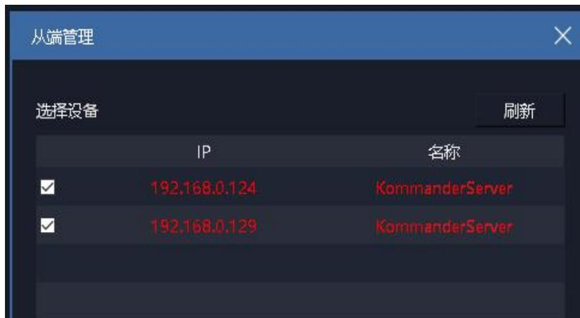
The abnormal color indicates that the connection with the slave terminal is abnormal, so that the master terminal cannot control the slave terminal. Maybe the experimental environment of the master-slave linkage has not been established, so the original white IP address and name become red. We can check the following conditions:
