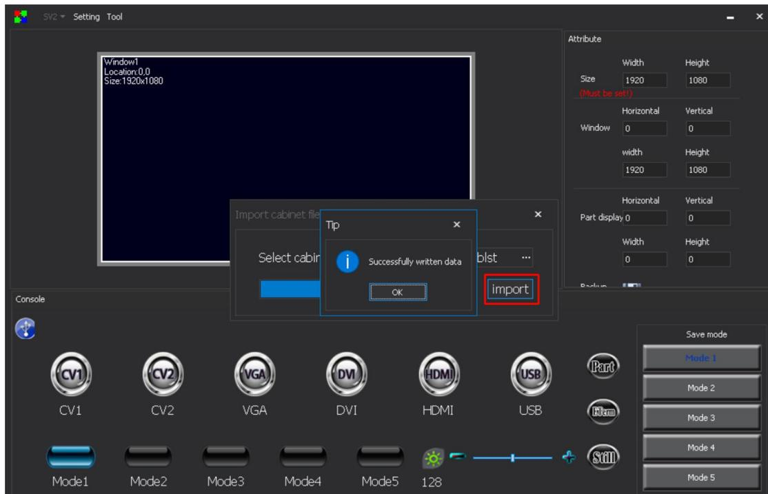
After the software prompts that the data is successfully written, it can be debugged by the video processor. When the processor selects the box file, the imported file will be displayed on the LCD screen.
