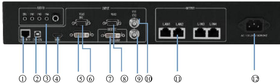
1、 UART-----Connecting PC Software through 9-pin Serial Port to RJ45 Network Port
